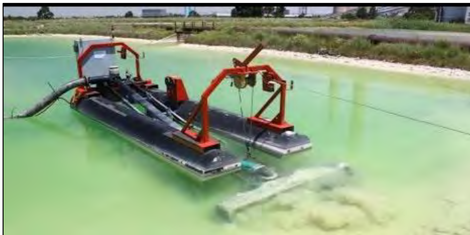
Figure 5-2. S.A.M.E. auger dredging, Australia
