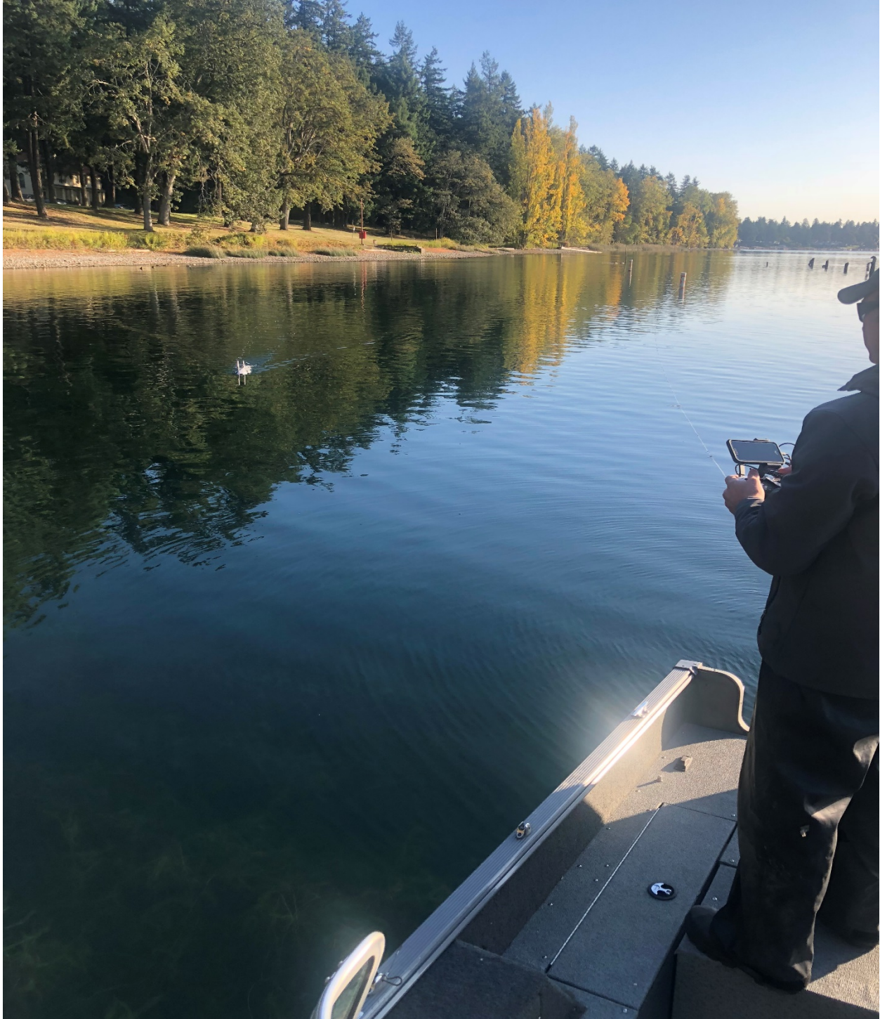
Aquatechnex biologist deploying 4k video drone system. This system has 4K resolution camera, is controlled by handheld system and is steered to locations to video or runs programed transects.
