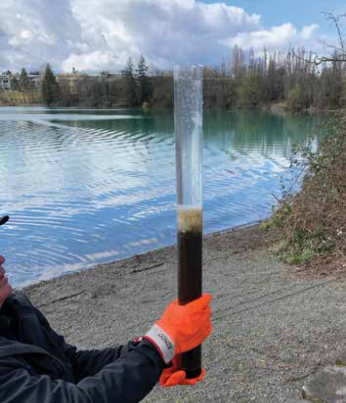
A sediment core sample taken from the lake after treatment. Alum is visible on top of the sediment. The water above the alum layer is clear and filled nearly to the top of the container.
