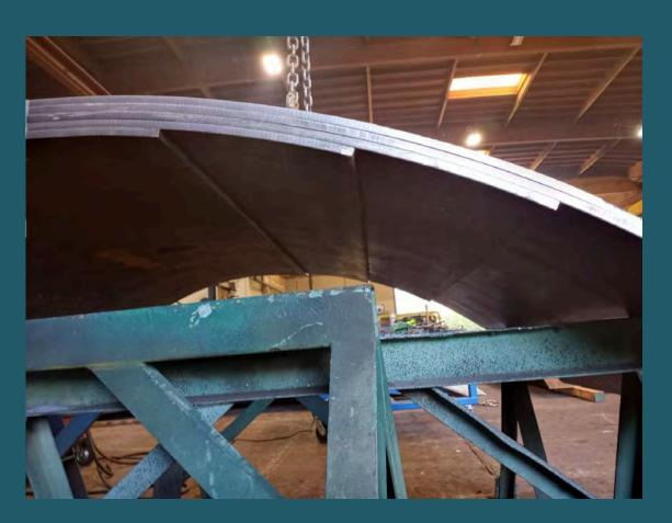
Sculptures rolled from long narrow steel blades into graceful curves. Shop in Portland that can roll 3" thick steel plate
