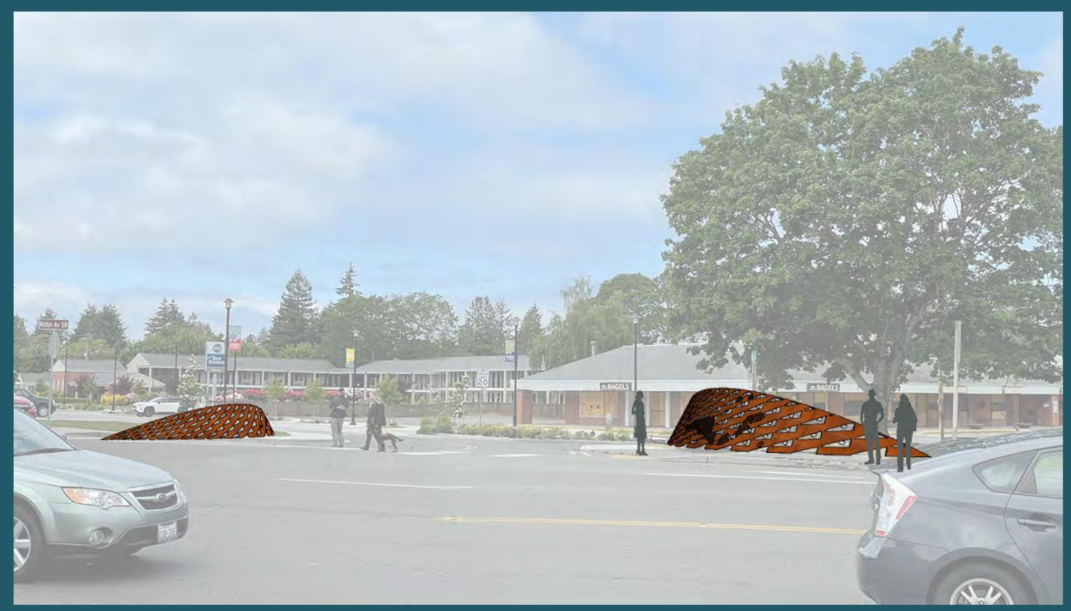
The smaller Arc on the south side is 32' long by 4' tall. The larger northern *Arc* is 40' x 7'-6". Each arc is rolled from 1-inch thick mild steel.
