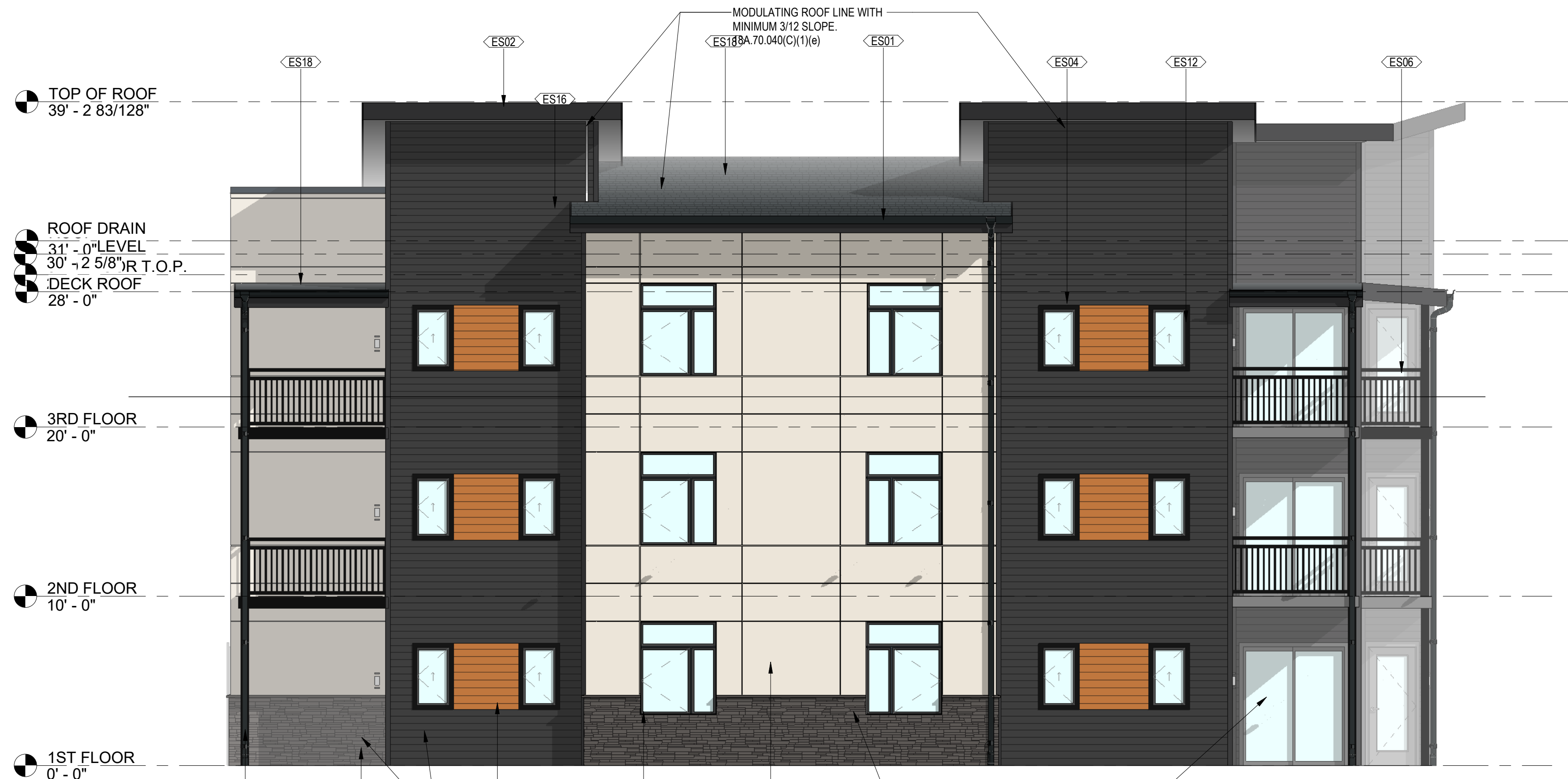
1 | DESIGN REVIEW - SOUTH ELEVATION 3/16" = 1'-0" CHANGES IN BUILDING MATERIAL WITH EACH PLANE 18A.70.040(C)(1)(d)(v) DISTINCTIVE WINDOW PATTERNS EQUAL TO ARTICULATION INTERVAL 18A.70.040(C)(1)(f)(i)
