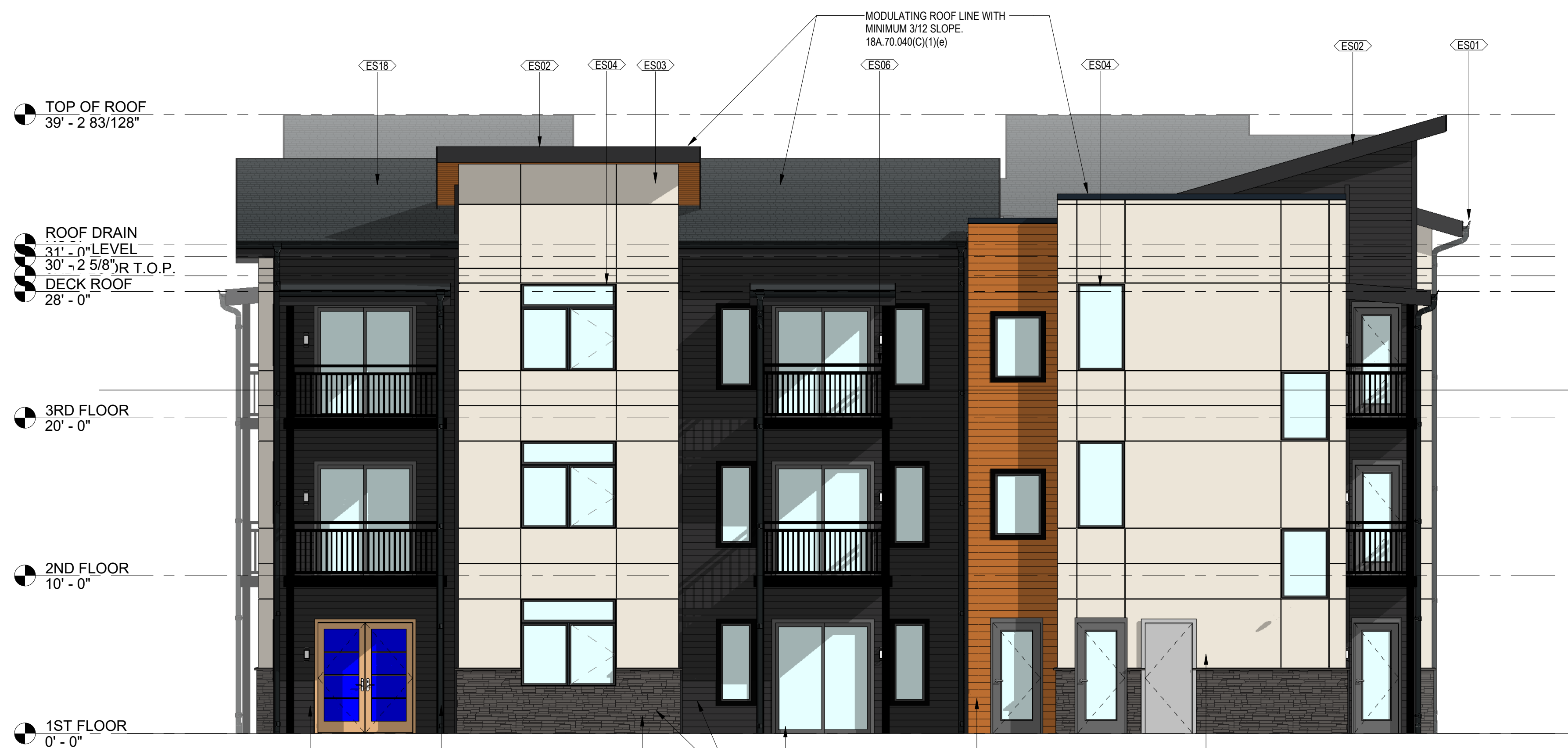
2 | DESIGN REVIEW - WEST ELEVATION 3/16" = 1'-0" CHANGES IN BUILDING MATERIAL WITH EACH PLANE 18A.70.040(C)(1)(d)(v)
