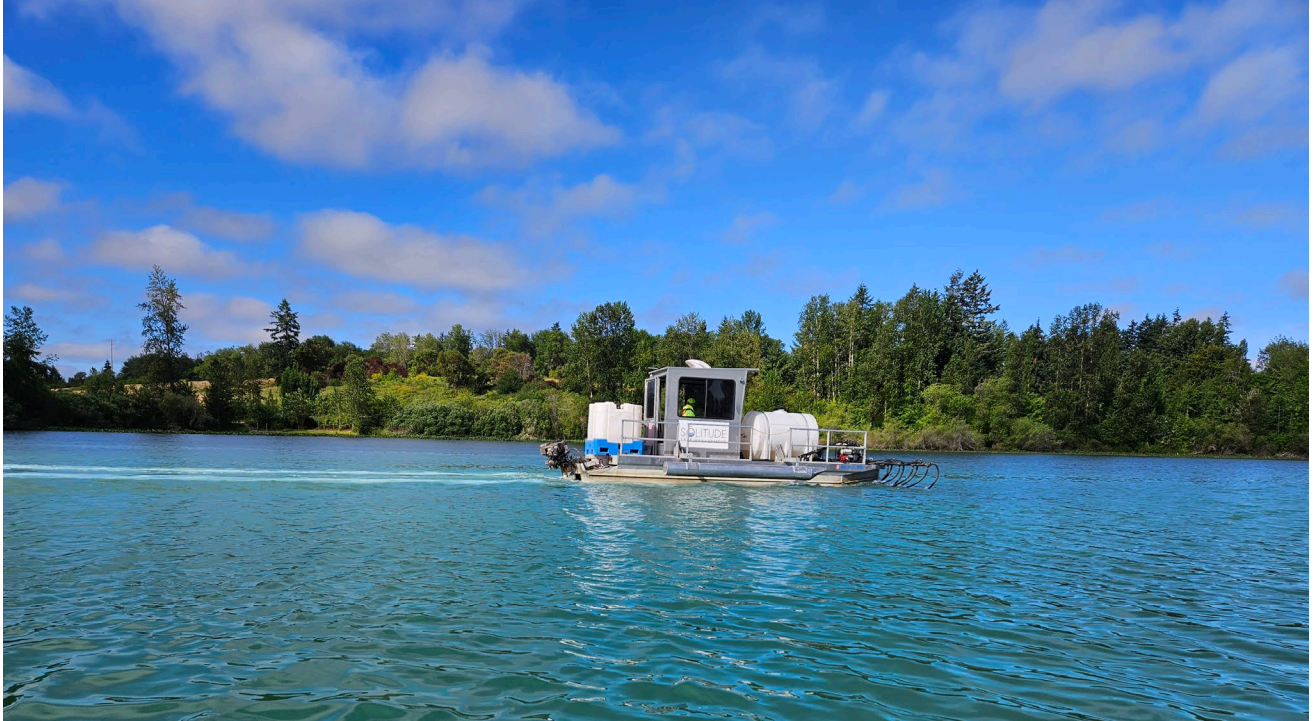
Figure 3. Alum barge during application on second day of treatment in June 2023
