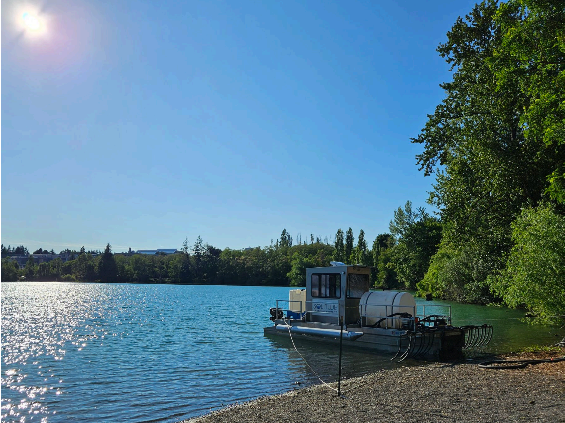
Figure 2. Chemical distribution system for 2023 alum treatment in June
