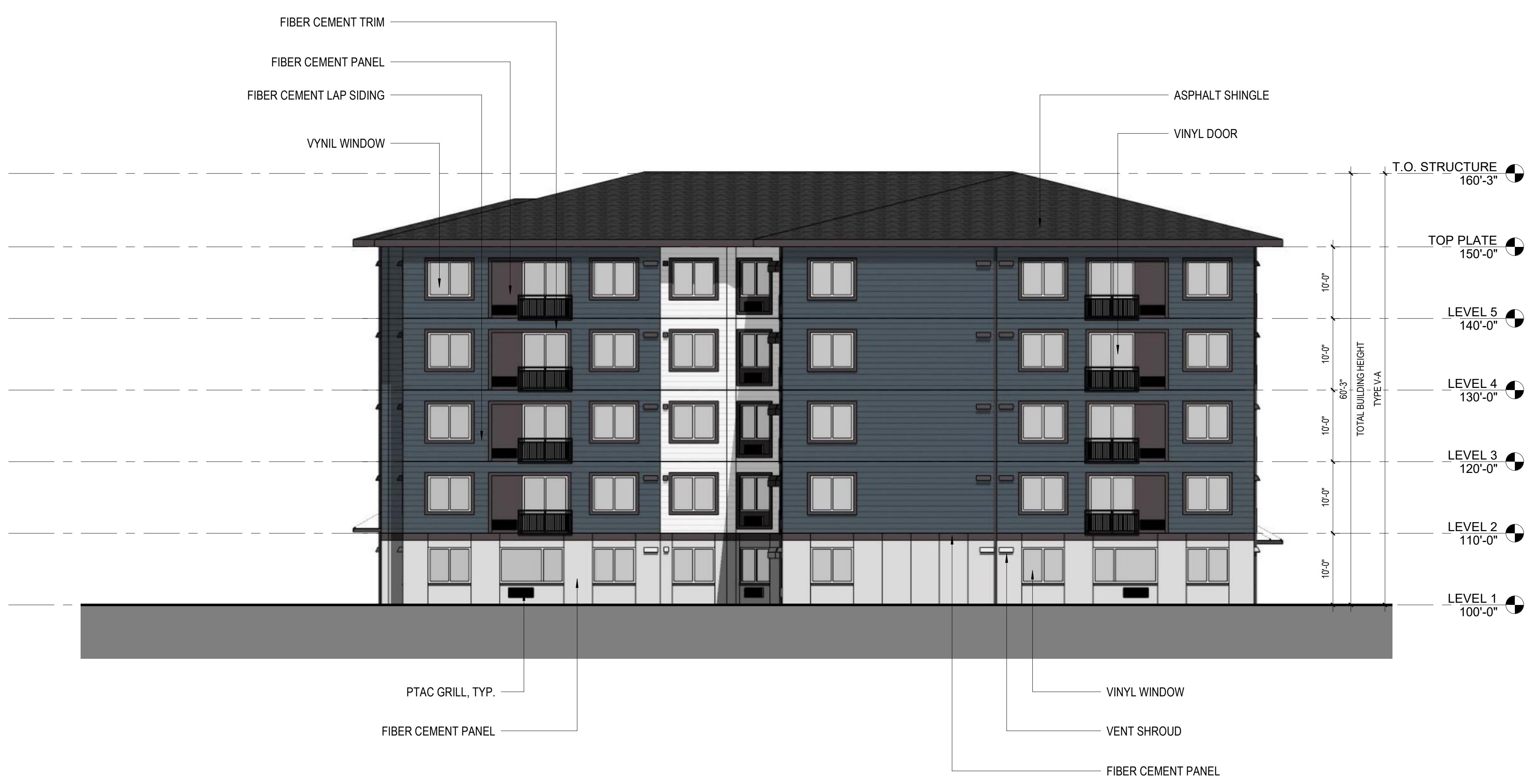
2 E3.04 BUILDING ELEVATION - EAST BUILDING B - WEST 1" = 10'-0"
