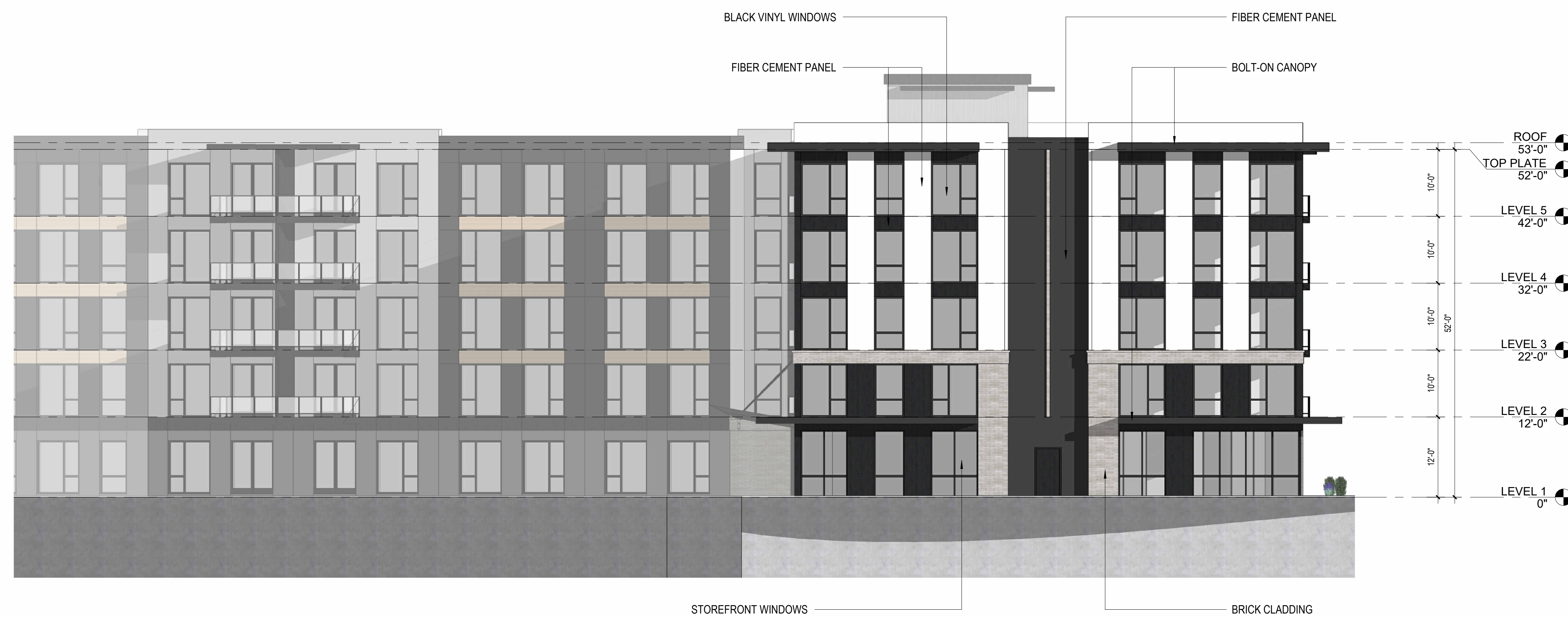
3 W3.01 NORTH ELEVATION (WEST WING) 1" = 10'-0"
