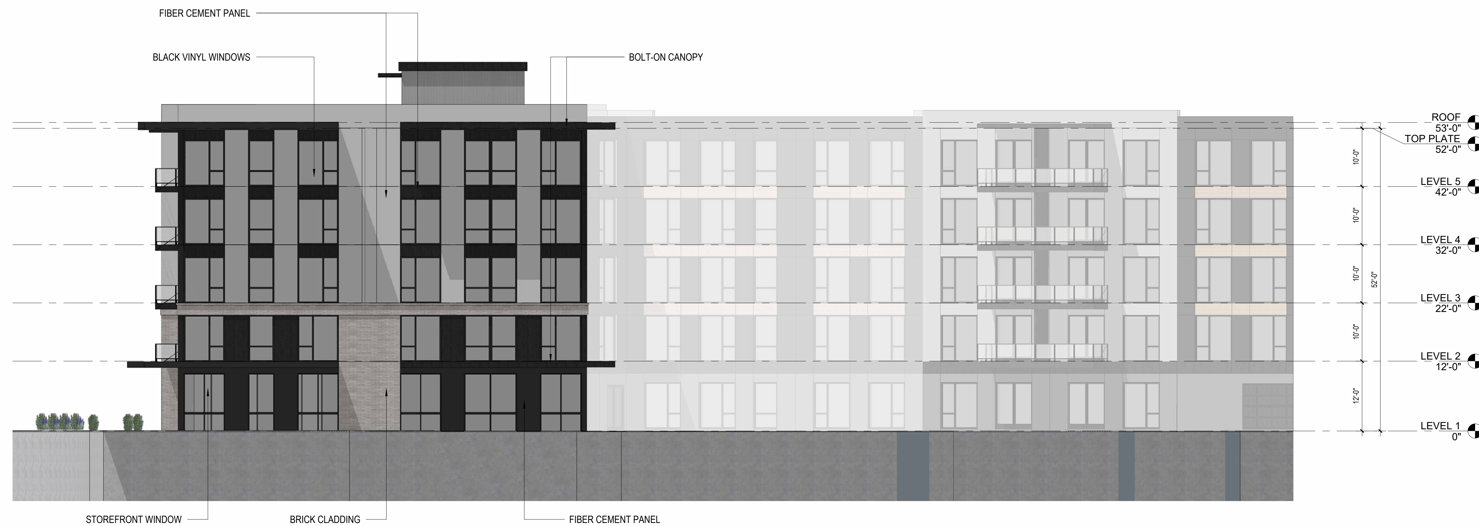
1 SOUTH ELEVATION (WEST WING) W3.04 1" = 10'-0"
