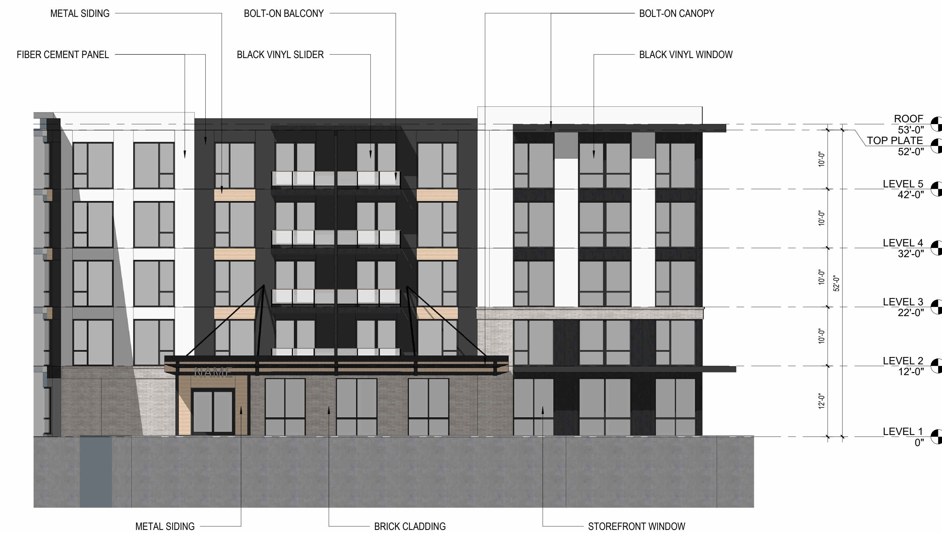
1 MAIN ENTRANCE ELEVATION W3.03 1" = 10'-0"
