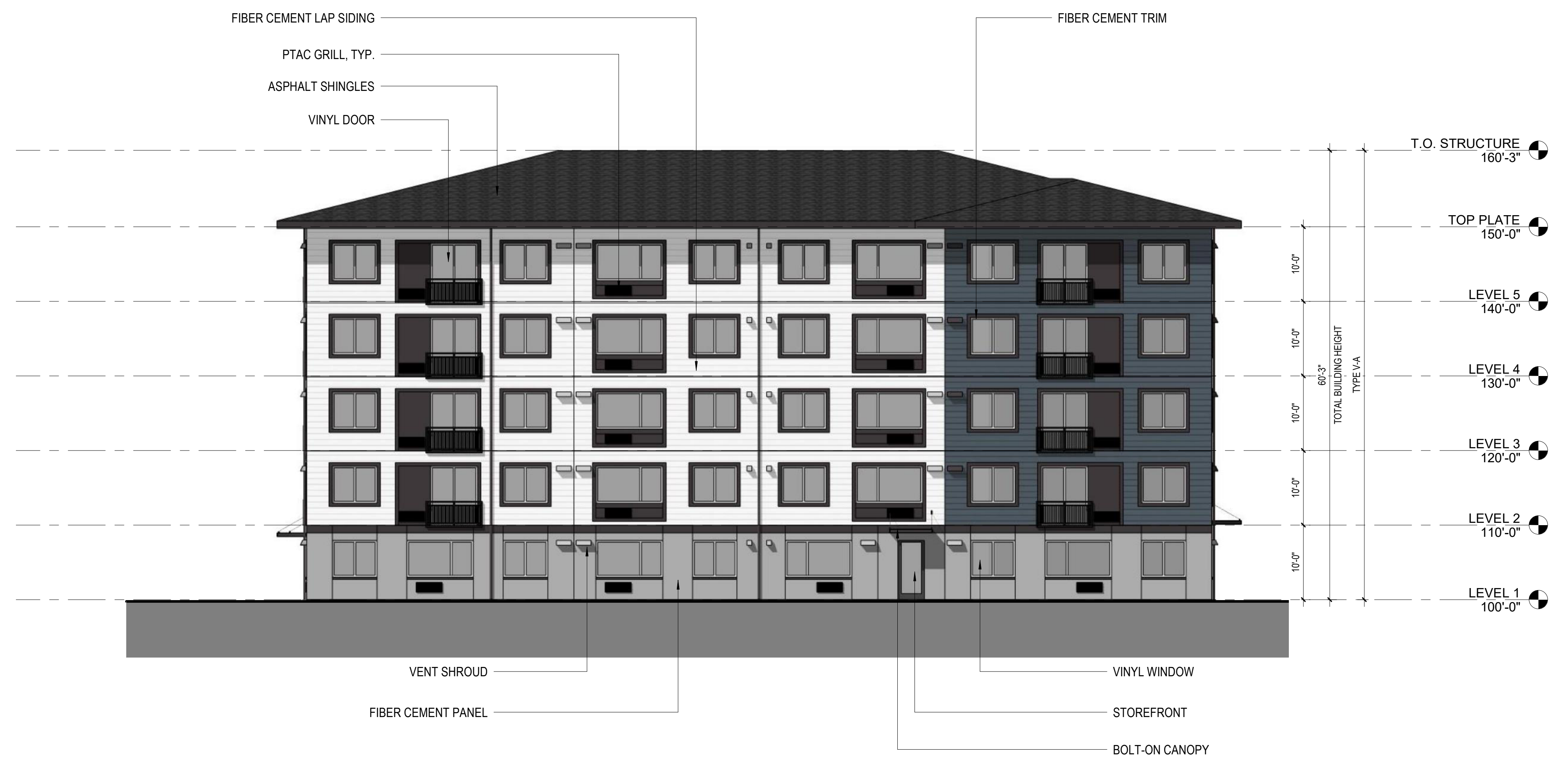
2 BUILDING ELEVATION - EAST BUILDING B - EAST E3.03 1" = 10'-0"
