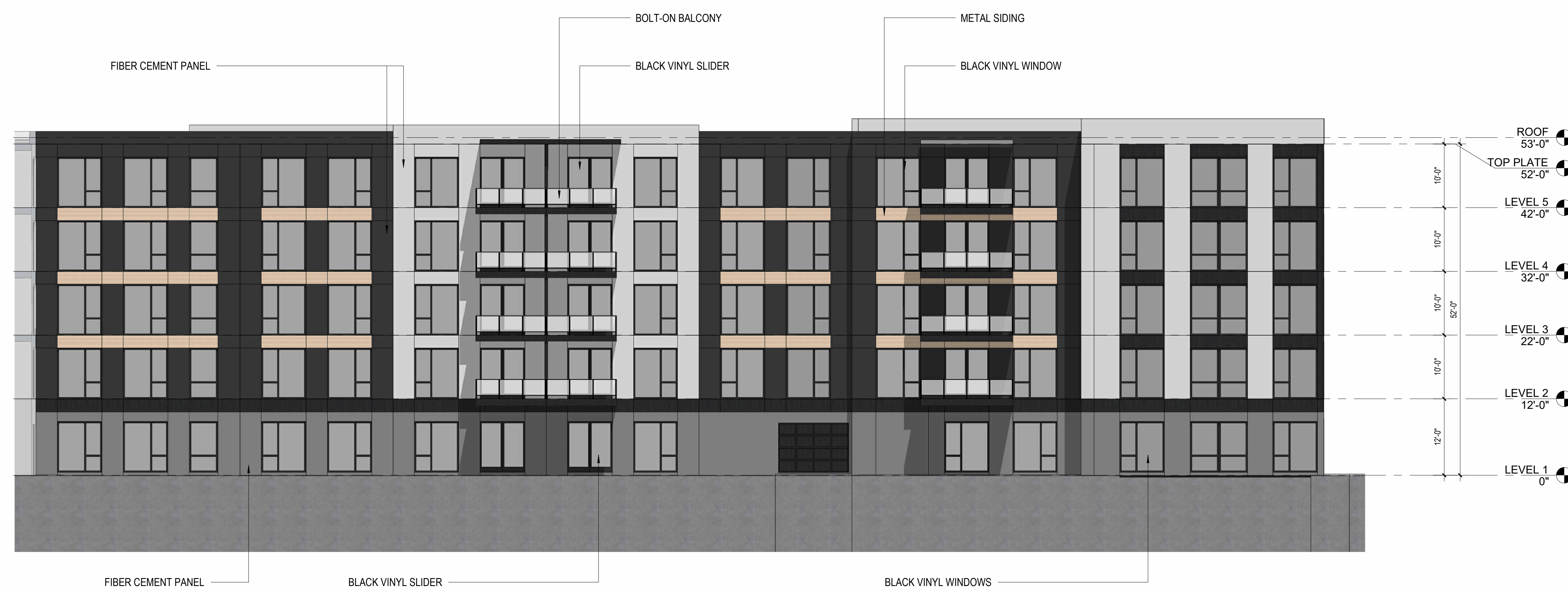
2 SOUTH ELEVATION W3.02 1" = 10'-0"
