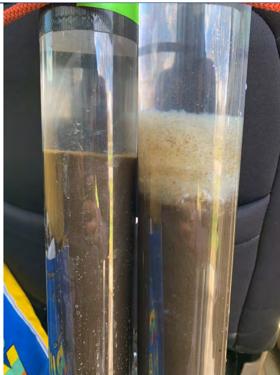
Figure 31. Sediment core collected prior to treatment on March 23, 2020 (left) and sediment core collected immediately following treatment on March 25, 2020 (right) with visible alum floc layer.
