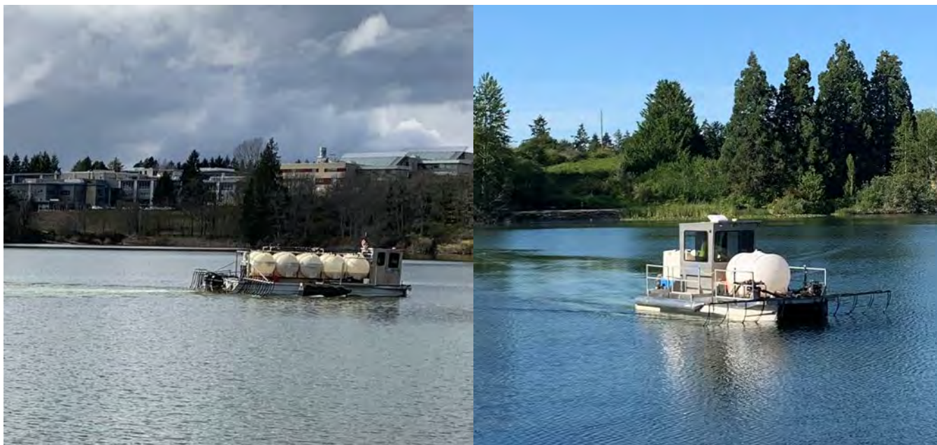
Figure 4. Chemical distribution systems for 2020 alum treatments in March (left) and July (right) at Waughop Lake.
