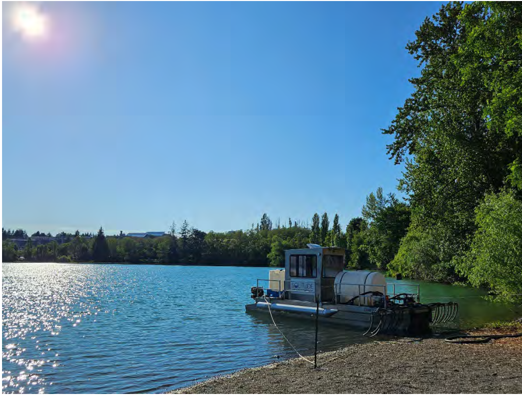
Figure 6. Chemical distribution system for 2023 alum treatment in June at Waughop Lake.
