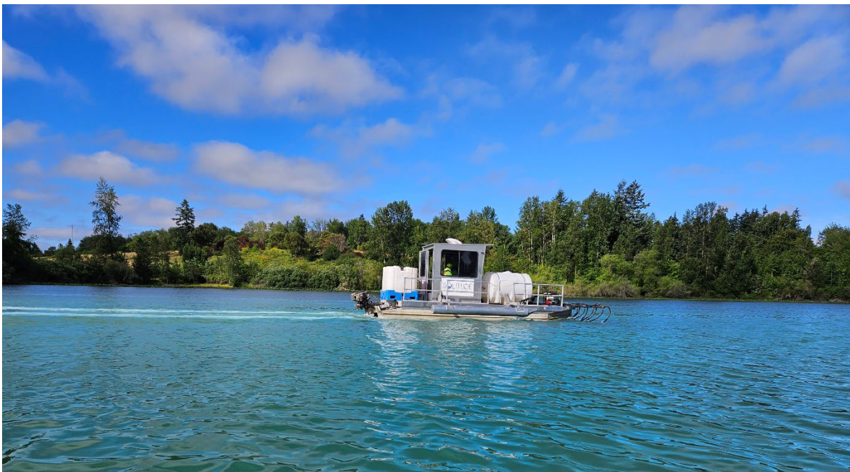
Figure 7. Alum barge during application on second day of alum treatment in June 2023 at Waughop Lake.
